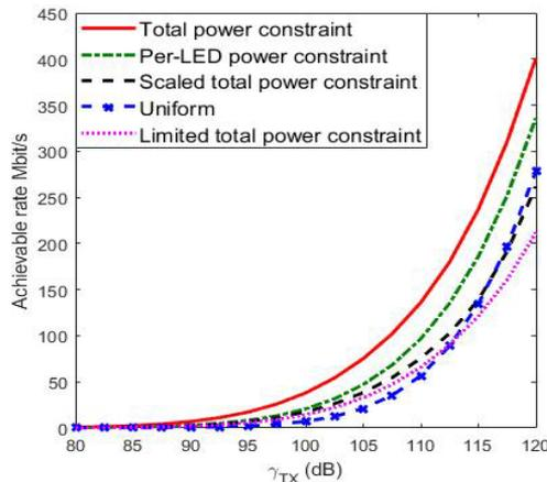
Figure 2: Throughput achieved by a 4x4 LED-based D-MIMO OWC system in the considered scenario.
