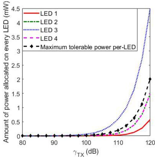
**Figure 3: Amount of power allocated on every LED when performing a power allocation optimization under a total power constraint.**
