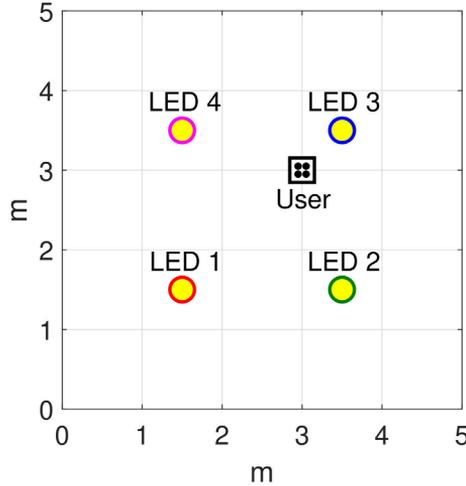
Figure 1: A 4x4 LED-based D-MIMO OWC system with an user placed close to one of the LEDs.
