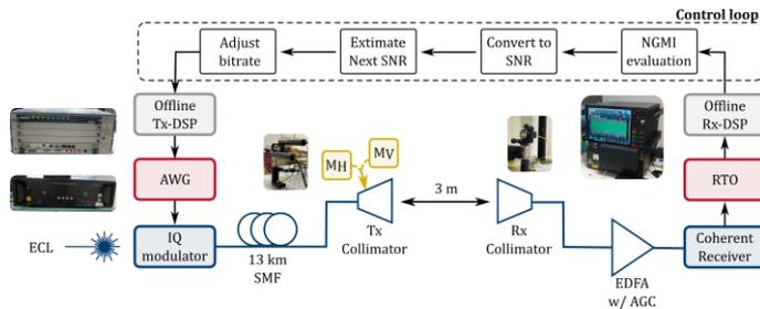
**Fig. 1 - Experimental setup of a coherent fiber-OWC link capable of transmitting 1 Tbps.**
