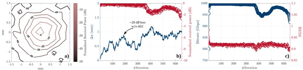
**Fig. 2 - Experimental results: a) calibration of the received power in function of beam deviation; b) received power with the AGC-EDFA for a random positional noise; c) transmitted bitrate and NGMI depending on the beam misalignment.**
