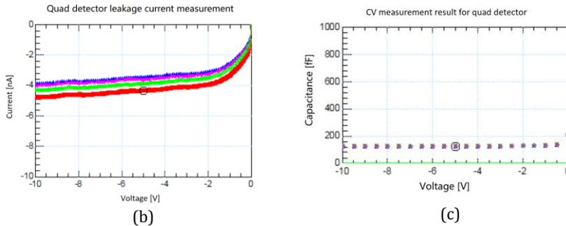
**Fig. 1 (a), Top, Schematic of a large-area quad photoreceiver. (b), bottom left, leakage current measurement result of 4 quadrants under different reverse bias voltage (c), bottom right, CV measurement shows capacitance of each quadrant around 123.5 fF**
